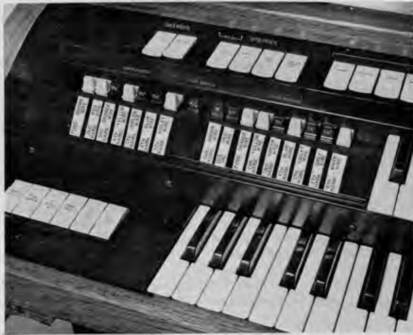
Figure 1-7. Tonebars and Control Tabs (Partial View)
