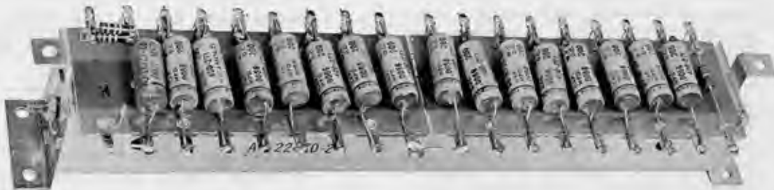
Figure 2-3. Vibrato Line Box
