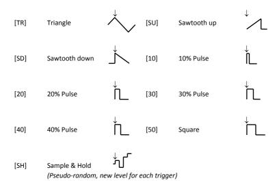
Sets the waveshape of the LFO. All waveshapes modulate CV and/or Aux 1 to any value between 0 to a positive value except triangle, which modulates positive and negative. The downward arrow indicates the default start point, which can be changed with Parameter 53.
