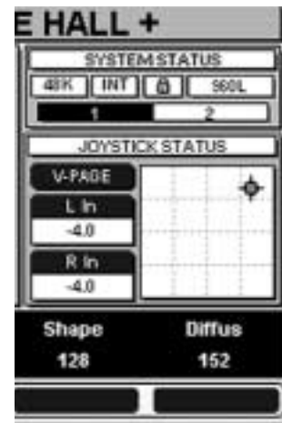
Figure 3-6 — JOYSTICK STATUS Display
