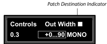
The Out Width value will be changing from 0 to 90 and back again.
