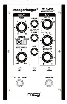
**DRIVE Control** - Sets the input sensitivity of the Cluster Flux. This control is only active when the Effect is on. The available gain is from -7dB to +28dB nominal. The Cluster Flux is designed to work with instrument or line-level signals.
