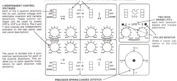
The perfect synthesizer controller. When released, it automatically snaps back to zero vertical position. When offset from this position, the modulation depth selected in each of the four possible directions is directly proportional to the amount of offset.
