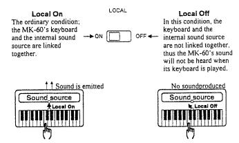
Local Off is effective to use when you wish only a connected module to be sounded, or when you have a MIDI sequencer connected.
