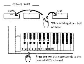
\* Once a receive channel has been set, the unit enters the Omni Off mode.
