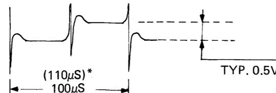
Mixing two outputs from BBD enables elimination of the clock component. For more precise adjustment, change the value of R52 or R53.
