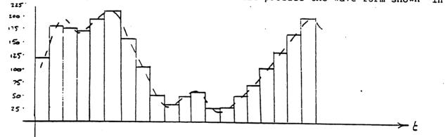
With the addition of filtering, a fairly accurate representation of the original wave form is produced. (Dotted line).
