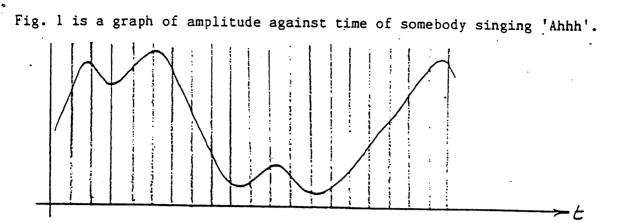
The amplitude of the signal can be represented by a number and if the wave form is measured at regular intervals these numbers would represent the change in amplitude of the signal over time.
