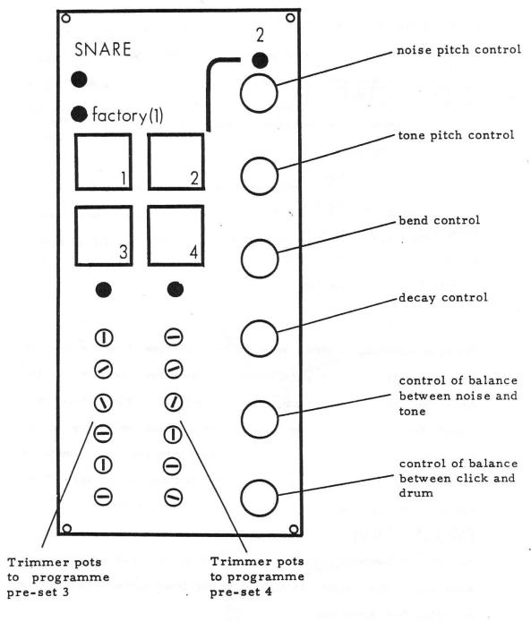
The trimmer pots have the same effect on pre-sets three and four as the controls on the right of the module have on pre-set No. 2. Their positions relate exactly to the controls -- i.e. noise pitch at the top through to click-drum balance at the bottom.
