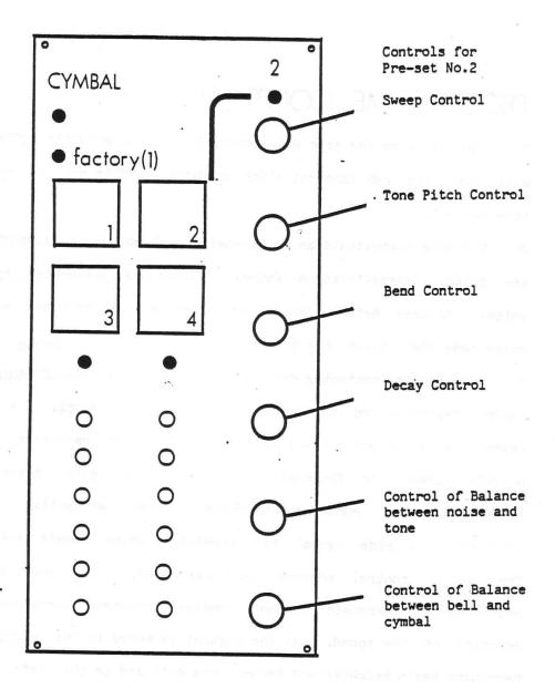
The trimmer pots have the same effect on pre-sets three and four as the controls on the right of the module have on pre-set number two. Their positions relate exactly to the controls - i.e. sweep at the top through to bell cymbal balance at the bottom.
