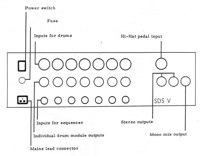
The rack is of standard 19" format and contains the power supply and input and output circuitry to take up to seven drum modules. It also contains a module for individually controlling the sensitivity and output of up to seven modules.
