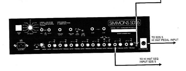
When CH 8 is used to open/close the Hi Hat, information entered has a different effect. Instead of giving a short pulse for every light in the matrix, CH 8 sends a 'pedal open' signal to the SDS 5. If no lights are on in CH 8 then the Hi Hat is permanently closed.
