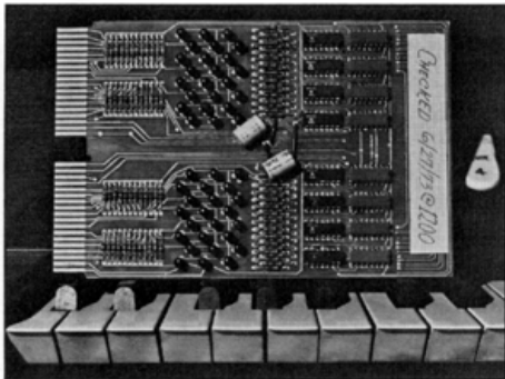
A key circuit from Knowlton's interface system.
